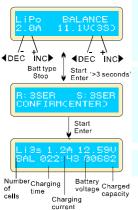
The left side of the first line shows the type of battery you choose. The value on the left of the second line of the charger is current user set, After setting the current and voltage, press START/ENTER key for more than 3 seconds to start the process.(charge current: 0.1-5.0A, voltage: 1-5V).
