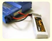
The main battery leads must be connected along with the balance lead connector as shown before charging your battery  $\dots$
