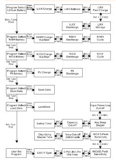
As default this charger will be set to typical user settings when it is connected to a 12V battery for the first time. The screen displays the following information in sequence and the user can change the parameter on each screen.
