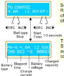
Set up the charge current on the left and nominal voltage on the right. Range of current is 0.1-5.0A, the voltage should match the battery being charged. Press START/ENTER key for more than 3 seconds to start charging.
